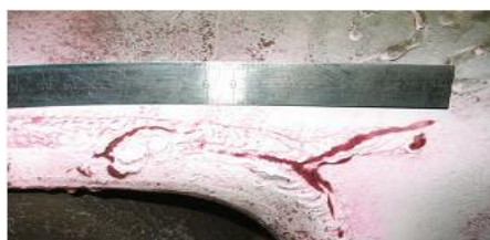
Figure 4 – Results of control by getting substances (CGS) in the field of axle-box knot
